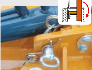
Perno per blocco meccanico in trasporto, (no catene, no staffe). Mechanical locking pin for transportation, (no chains, no brackets).
