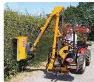
T320A/R Versione per trattori con guida reversibile. For front mounting on tractors with reversible drive.
